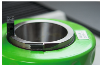
Spindle with integrated calibration edge
